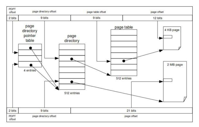
The top half of the figure shows how the processor translates a virtual address to a physical address by using the normal, three-level, paging scheme:
